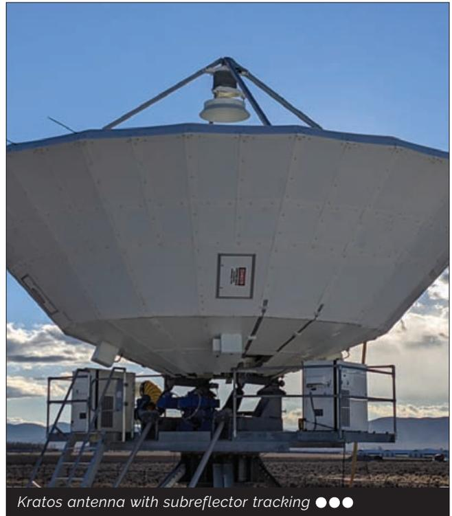
Kratos antenna with subreflector tracking ●●●
