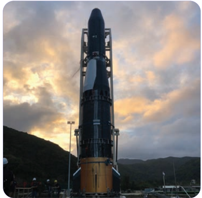
HAPITH V launcher can lift a 390kg payload to LEO and 350kg payload to SSO
