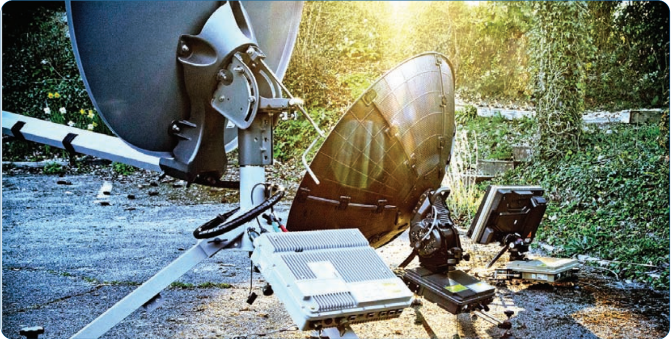
Satcom terminals integrated with the PIM. Photo courtesy Paradigm Communication Systems
