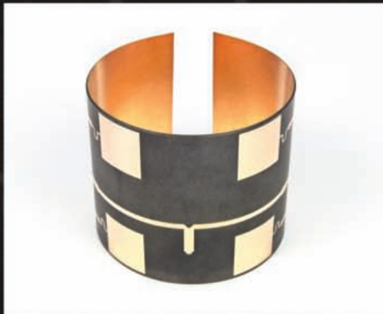
Right: 2D radiation patterns Below: Curved Antenna showing radiation patches.
