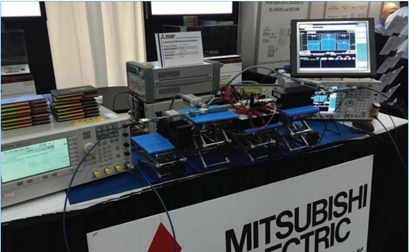
Mitsubishi Electric US, Inc. - At EDI CON in September 2016, Mitsubishi Electric US, Inc. presented a hands-on live demonstration of its latest cutting edge GaN technology. A "mini-lab" was set up at the company's booth showcasing its latest linearized 2-stage 70W Ku-band evaluation board. With improved gain and efficiency compared to earlier process generations, this compact design provides 40-45 watts of linear power with more than 30dB gain and combined efficiencies >20% across the 13.75-14.5GHz band, allowing customers the ability to design more competitive, highly scalable SSPA and BUC products. ●●●
