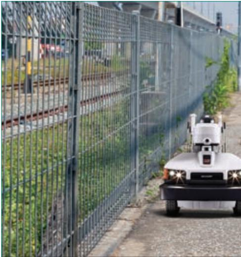
● ● Sharp INTELLOS Automated Unmanned Ground vehicle (A-UGV)
