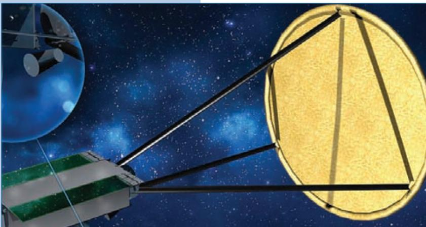
The antenna is constructed with a lightweight shape memory polymer (SMP), which means it can be folded up like a parachute for launch ●●●
