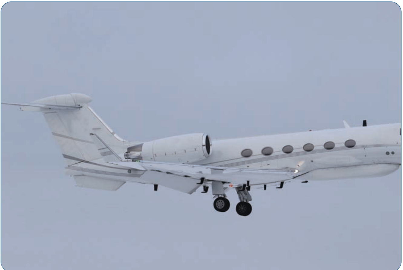
A Government Gulfstream FlexAir Tail Mount 45cm 18" Antenna. Gulfstream aircraft are in use today for enroute comms, ISR and VIP applications.
