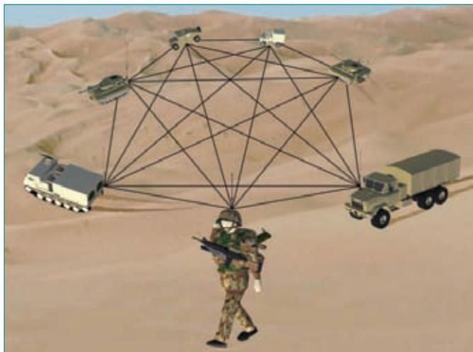
● ● Figure 5. Mesh Networks that can be rapidly simulated using the Quintech NEXUS matrix switch a) Full Mesh
