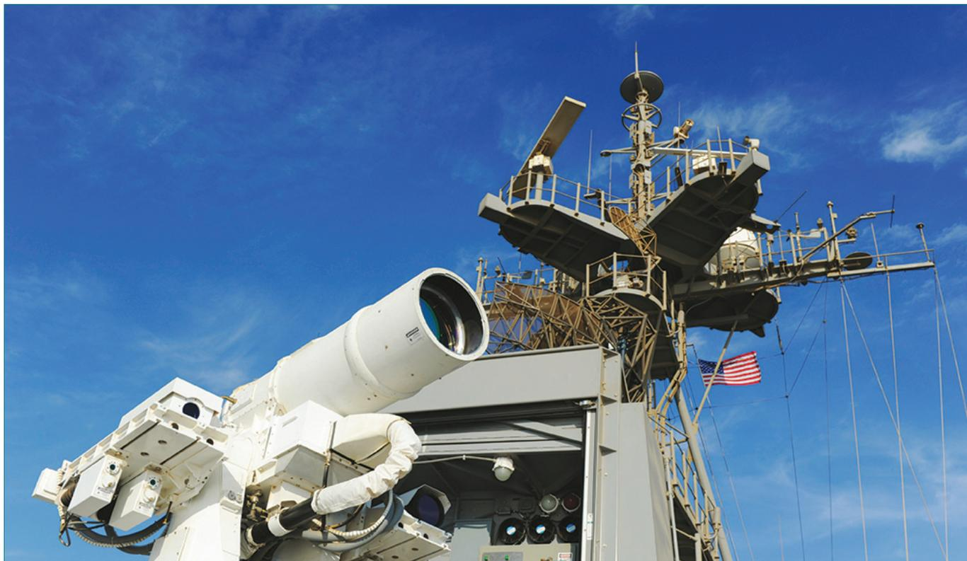
● ● Active laser deployed on the USS Ponce amphibious transport ship. Video/ image courtesy of CNN/US Navy
