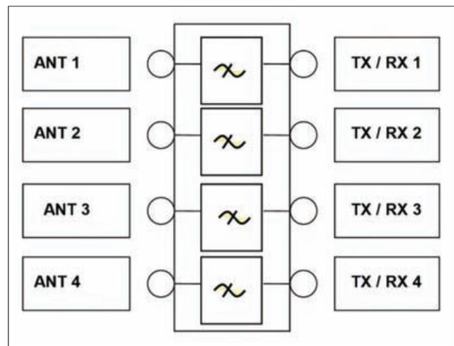
Figure 2: Block diagram of quad bandstop filter ●●●
