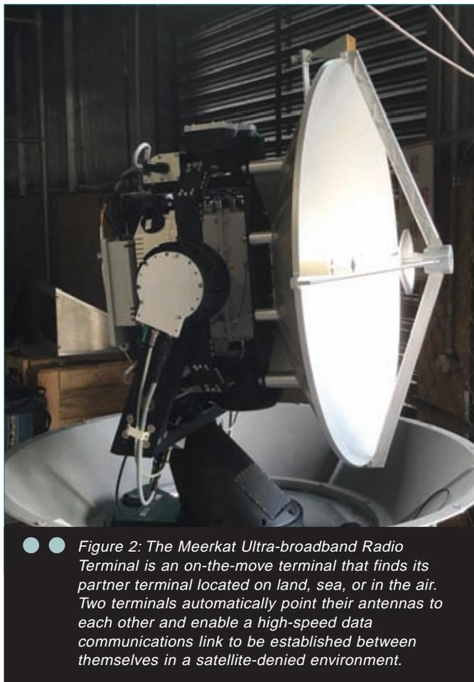
● ● *Figure 2: The Meerkat Ultra-broadband Radio Terminal is an on-the-move terminal that finds its partner terminal located on land, sea, or in the air. Two terminals automatically point their antennas to each other and enable a high-speed data communications link to be established between themselves in a satellite-denied environment.*
