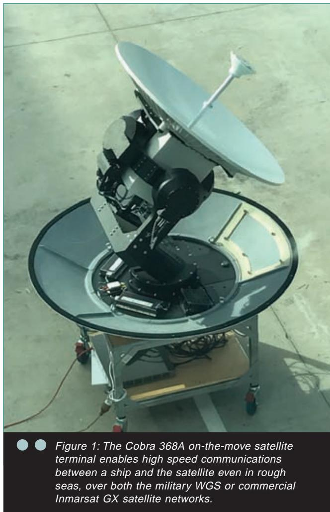
● ● *Figure 1: The Cobra 368A on-the-move satellite terminal enables high speed communications between a ship and the satellite even in rough seas, over both the military WGS or commercial Inmarsat GX satellite networks.*
