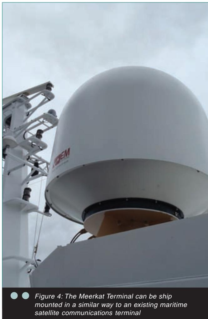
● ● *Figure 4: The Meerkat Terminal can be ship mounted in a similar way to an existing maritime satellite communications terminal*
