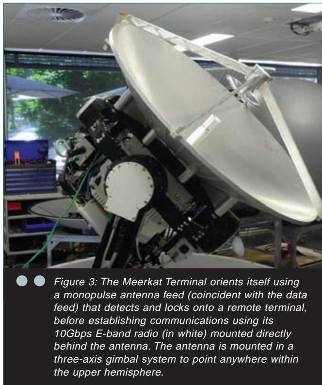
● ● *Figure 3: The Meerkat Terminal orients itself using a monopulse antenna feed (coincident with the data feed) that detects and locks onto a remote terminal, before establishing communications using its 10Gbps E-band radio (in white) mounted directly behind the antenna. The antenna is mounted in a three-axis gimbal system to point anywhere within the upper hemisphere.*
