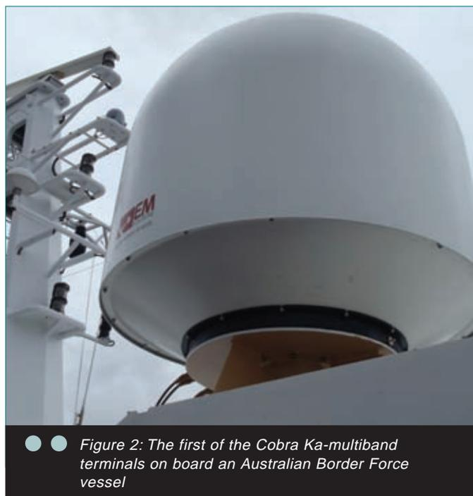
● ● *Figure 2: The first of the Cobra Ka-multiband terminals on board an Australian Border Force vessel*
