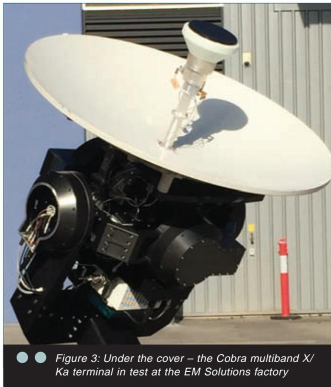
● ● *Figure 3: Under the cover – the Cobra multiband X/Ka terminal in test at the EM Solutions factory*
