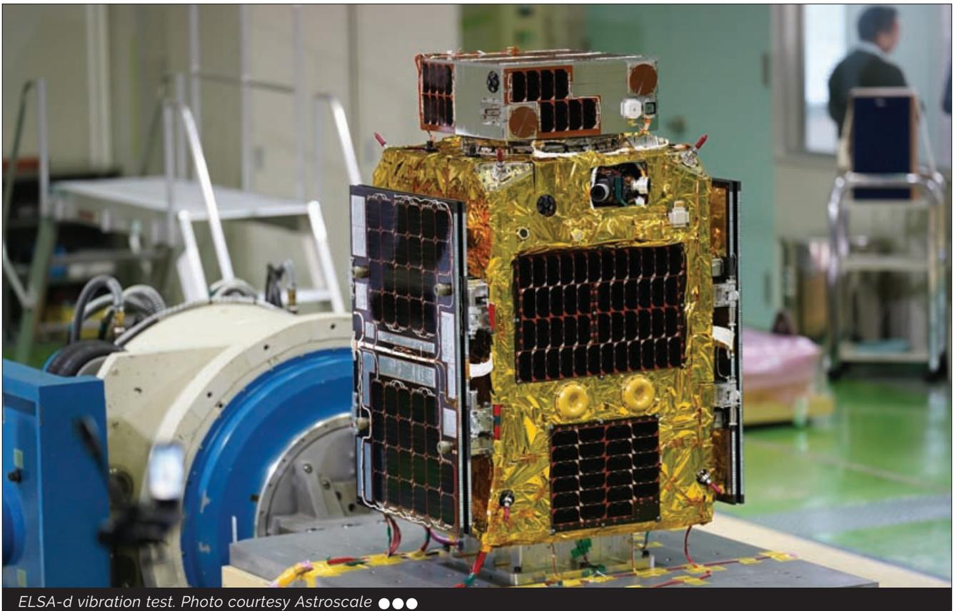
ELSA-d vibration test. Photo courtesy Astroscale ●●●
