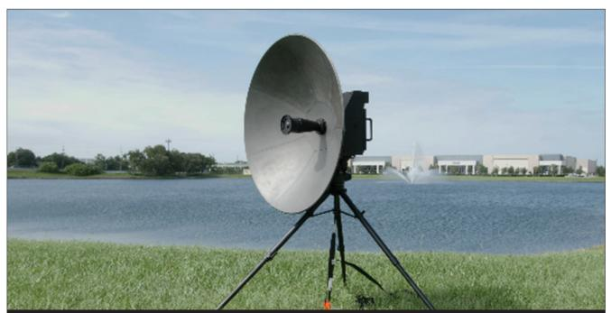
Mobile by design, and the smallest of Comtech's Family of Troposcatter Systems. Comtech's Compact Over-the-Horizon Transportable Terminal (COMET™) is the world's smallest and lightest modular, man-packable troposcatter system. COMET was developed to provide resilient communications in contested environments addressing a wide range of tactical mission needs. Photo courtesy Comtech ●●●
