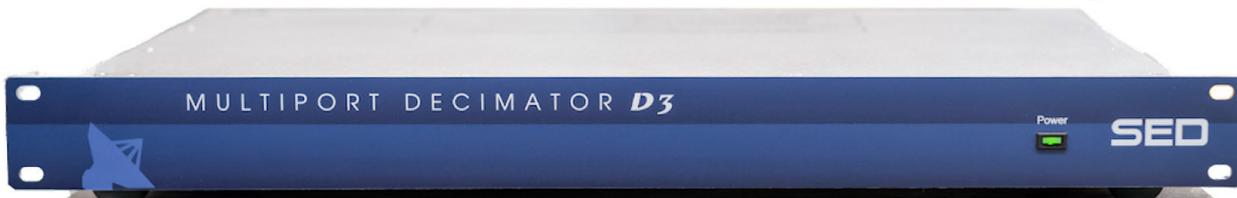
SED's Multi-Port Decimator D3 is a third generation spectrum measurement and analysis unit in a 1U chassis with an integrated 8-port RF switching capability. It is ideal for either local or remote monitoring of multiple feeds and carriers in satellite, cable or terrestrial wireless networks.
