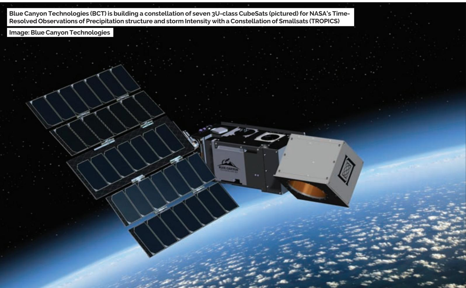
smaller spacecraft built in a new way. Not the lengthy bespoke process of building a multi-tonne spacecraft destined for geostationary orbit, but using a combination of off-the-shelf components, new satellite system miniaturisation technologies, and mass-production techniques, at low-cost per-unit of functional capability.
