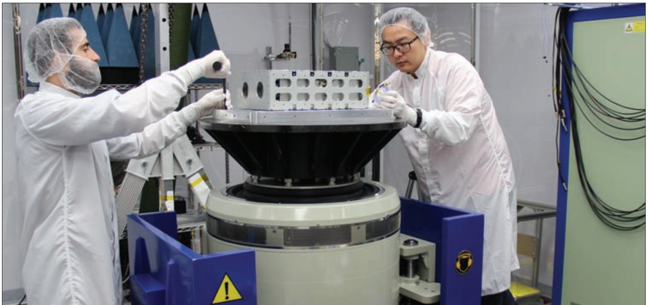
Kepler test model is prepared for vibration testing at Space Flight Laboratory in Toronto. Photo courtesy of SFL ●●●
